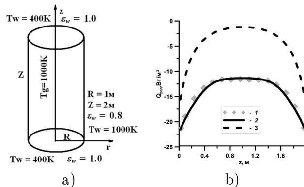
Fig. 4. A closed cylinder filled with a mixture of radiating gases: a) problem formulation; b) distribution of the radiation flux at the side wall of the cylinder: 1 – Yu et al., 2000; 2 – SigmaFW (FVM with WSGG); 3 – SigmaFW (FVM with then "grey gas" approach)
