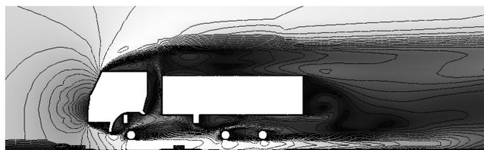
**Fig. 7.** Velocity field at flow around the vehicle by ram air
