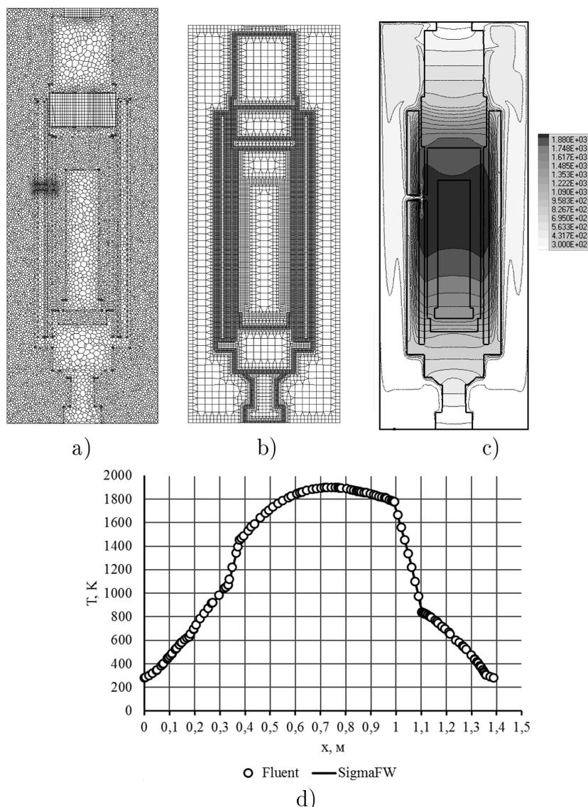
**Fig. 5.** Comparison of simulation results of a chemical reactor in terms of temperature fields. The calculation is performed using programs a) grid for "ANSYS"; b) grid for "SigmaFW"; c) temperature field, "SigmaFW"; d) distribution of temperature along the horizontal line passing through the hole
