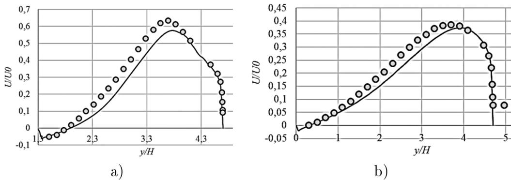
Fig. 3. The distribution of the longitudinal velocity component along the vertical lines at a certain distance. Points correspond to experimental data, while solid line shows calculation by SigmaFW: a) 13,5H; b) 27H from the inlet of the diffuser
