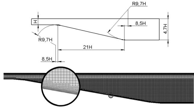
Fig. 2. Computational geometry with inlet and outlet section and the grid
