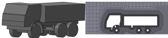
**Fig. 6.** Geometry and computational grid of the truck presented by the "SigmaFW" software package
