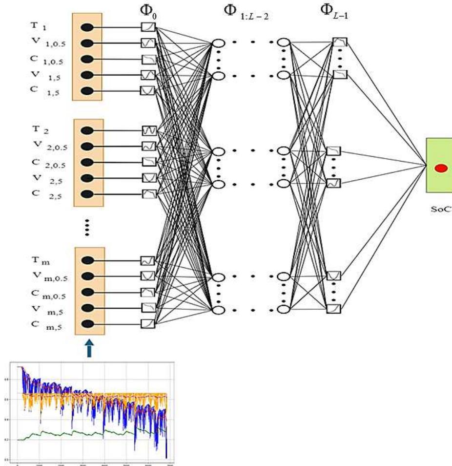
Fig. 1. KAN network architecture for State of Charge (SoC)
