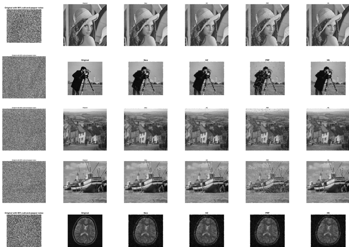
Fig. 3. First column: The noisy images with 90% salt-and-pepper, the original images (second column), third Column to last column: restored image by New method, HZ method, PRP method, HS method
